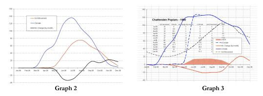
The SMD is represented by the solid blue line in the graph above. The effective climate values (those that influence root activity) appear as a broken blue line, commencing in May. The ground movement by month is plotted as a red line. The broken black line is cumulative ground movement, peaking around September and the ABA production phase is the red hatched shaded area.
