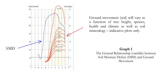
Alternatively, if the SMD values are particularly high then the tree will seek water quickly and trigger ground movement. A high SMD value in May, coincident with when a tree comes into leaf, will generate large tensile forces in the xylem and for this reason, 'sets the scene' which is then built on throughout subsequent months.
